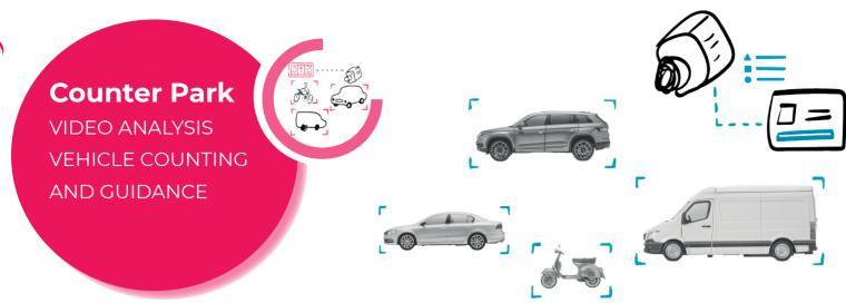
SIRAM COUNTER Park is a vehicle counting software based on Video Analysis. It identifies, classifies and tracks vehicles using deep learning algorithms that run directly on the camera.
